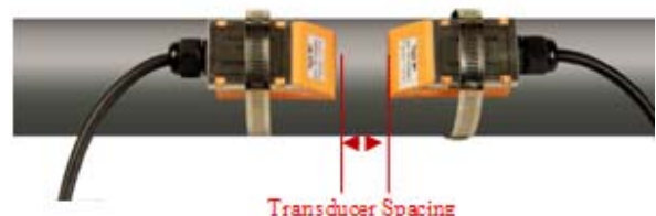
V-method clamp-on installation for standard temperature transducers (TM-1)
