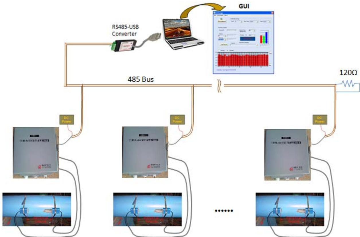
All the flowmeters are connected to a 485 bus which is then connected to data center computer. Each flowmeter has its own network address, so that the computer can query each flowmeter separately. The 120Ω terminator is needed when the 485 cable is long.
